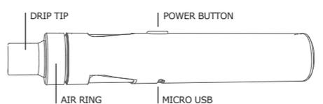
the resistance) and replace it with a new one, screwing it firmly. We suggest, before screwing the resistance, to soak the cotton inside with liquid for electronic cigarettes when the resistance is new. Maintaining the electronic cigarette Joyetech AIO in a vertical position, firmly tighten the metal ring previously unscrewed (inclusive of resistance). To refill with liquid the electronic cigarette Joyetech AIO with new resistance, follow the instructions under "modality of Use".
